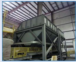
(2) 40 Ton Hoppers 12' x 12' x 14'H on Stands w/ Pneumatic Vibrators and conveyor
