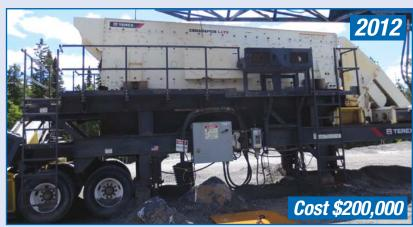
2012 Terex Model CRS 6203 Triple Deck Screen on T/A Trailer, s/n TRX6203SC0KCC0297 c/w Cedarapids Model LJ-TS ISH6203-32, 72" x 20' Triple Deck Screen, s/n IRX SC203 T DU C B 1258 w/ TWO 30" Finished Product Discharge Cross Conveyors.
