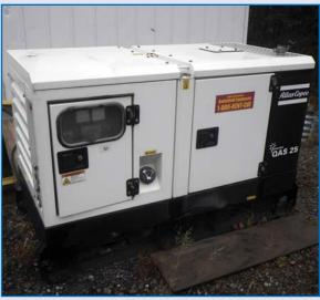
Atlas Copco Model QAS25KD-SKID, Skid Mount 20KW Generator, s/n H0P10097, 20KW/25KVA, 480/240/208V, 3 Phase
