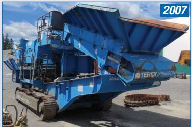
2007 Terex Pegson Maxtrak Model 1000MXT Crawler Cone Crusher, s/n 100568EF, w/ Caterpillar C9, 325 HP, BL Pegson Model 1000 Long Cone, 40", s/n QM034858 (Cone Main Bearing, Mantle and Liner changed approx. 20 Hours Ago), 38" x 16" Incline Feed Conveyor w/ Hopper & Metal Detector, 30" x 30' Cone Discharge Conveyor, Showing 8,500 Hour.
