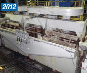
(4) 2012 Quinn Process Equipment Model QPEC #100 T-BR Flotation Machines c/w Double Froth Overflows and Froth Paddles with Drives & c/w Spencer Model 30103A3 Centrifugal Blower s/n 815558-F12
