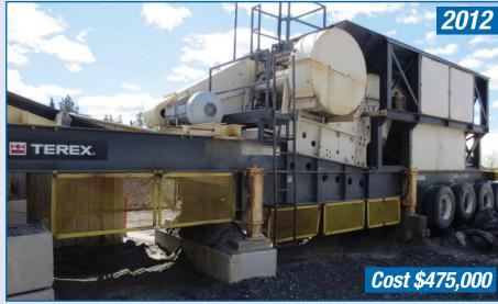
2012 Terex Cedarapids Model JS3042, 30" X 42" Jaw Crusher, s/n TRXJ3042POKCC w/ 150 HP Elec. Drive, Mounted on Quad Axle Hydraulic Levelling Trailer (p/w Honda GX 390 w/ hydraulic power pack) , s/n TRXJ3042POKCC0334 w/ Vibratory Feeder w/ Grizzly, 42"x 30' Outfeed Conveyor, Showing 2,700 Hours.
