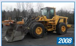
2008 Volvo L-180F Wheel Loader s/n UCEL18FH0011622, Showing 14,200 Hours, (Volvo Drop-In Engine Approx. 2,000 Hours Ago), 26.5R x 25 Tires
