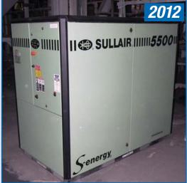
2012 Sullair S-Energy Model 5509AC, 75HP Screw Compressor w/ 125 PSI, 344 CFM, s/n 201209260054, Showing 6528 Hours
