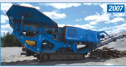
2007 Terex Pegson Model XR 400 Crawler Jaw Crusher, s/n 400258EFXR, w/ Caterpillar C9, 275 HP, 26" x 42" Jaw, 42"x 12' Vibratory Hopper Feeder w/ Grizzly, (Jaw s/n 0M055841), 36" x 32' Main Discharge Conveyor, 23" Fines Discharge Conveyor, 26" Tramp Steel Conveyor w/ Magnet, 20" Pads, Showing 7,600 Hours.
