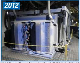
2012 Rotex Mineral Separator Model MM3180-3, 48' x 89" High Capacity, Twin Chamber Triple Deck Triplex Gyratory Screener, s/n SO 38597/0
