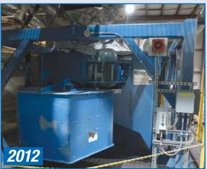
2012 Rotex Mineral Separator Model MM3180-2, 48' x 89" High Capacity, Twin Chamber Double Deck Triplex Gyratory Screener, s/n SO 38662/0
