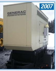
2007 Generac Model 8310670100, 100KVA, 600V Generator p/w Mitsubishi 4 Cyl. Diesel on T/A Carrier
